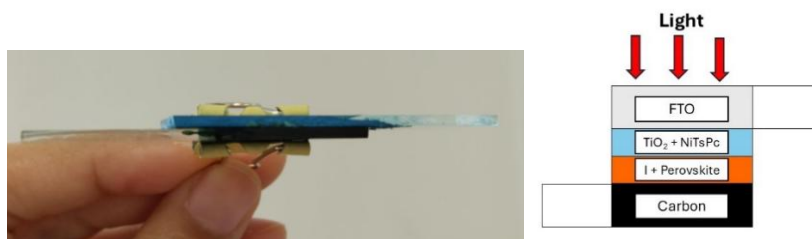
Figure 4: The attachment of surfaces of \text{TiO}_2 , NiTsPc, iodine, and perovskite onto carbon paste-FTO coated glass.
