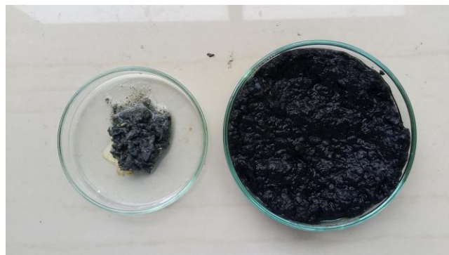
Fig. 4: Production of Immobilised Tyrosinase on Magnetic Chitosan (Left) and Magnetic Chitosan Gel (Right).
