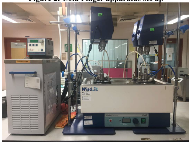
Figure 2: Cold Finger apparatus set up
