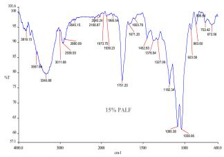
Figure 1: FTIR result for PLA + 15% PALF
