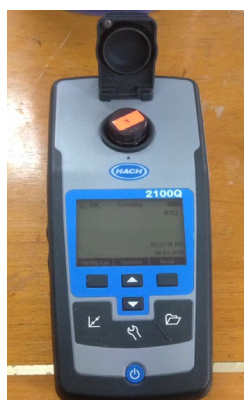
Figure 4: Turbidity meter 2100Q
