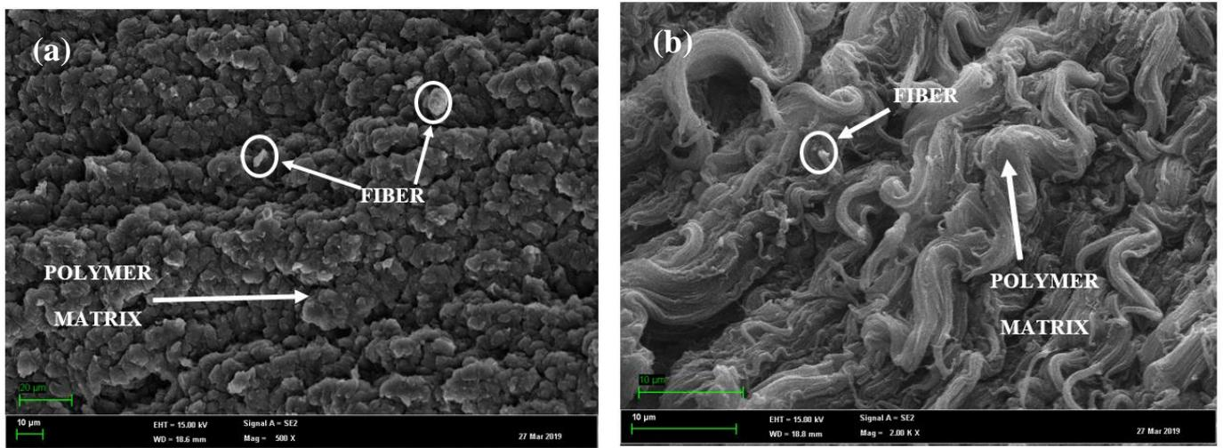
Fig. 3: SEM micrographs of the surface due to tensile stress (a)5wt% and 10wt% (b)15wt%
