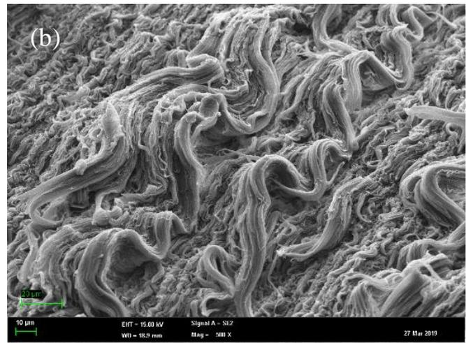
Fig. 1: SEM micrographs of (a) sample that is cut by liquid nitrogen and (b) sample that is cut due to tensile stress
