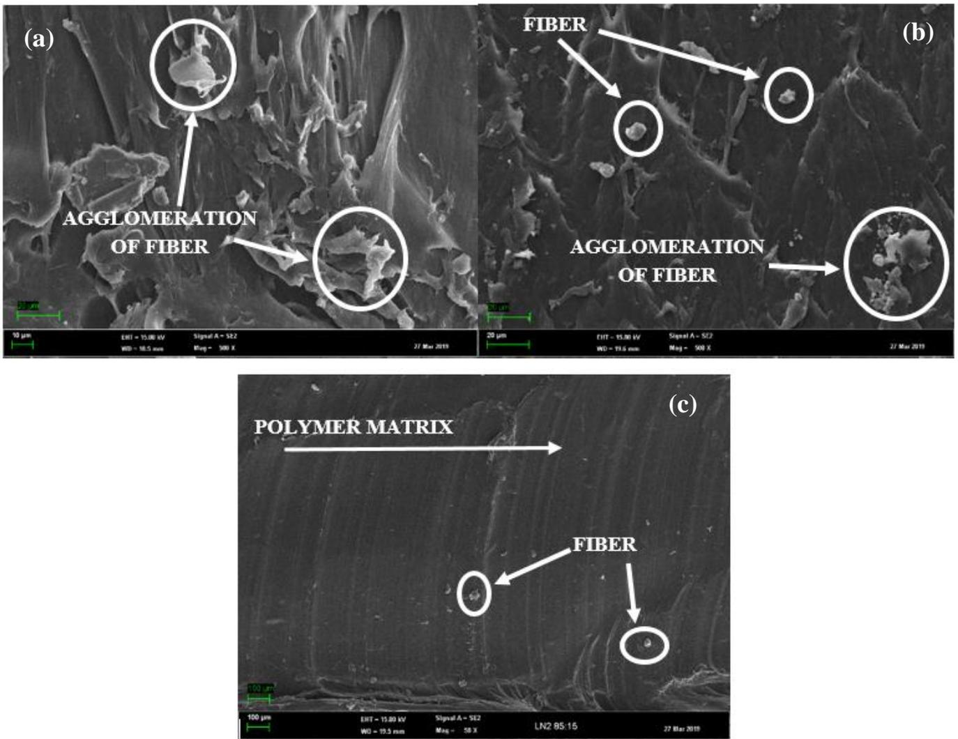
Fig. 2: SEM Micrographs of sample with different content of silica (a)5wt% (b)10wt% and (c)15wt%
