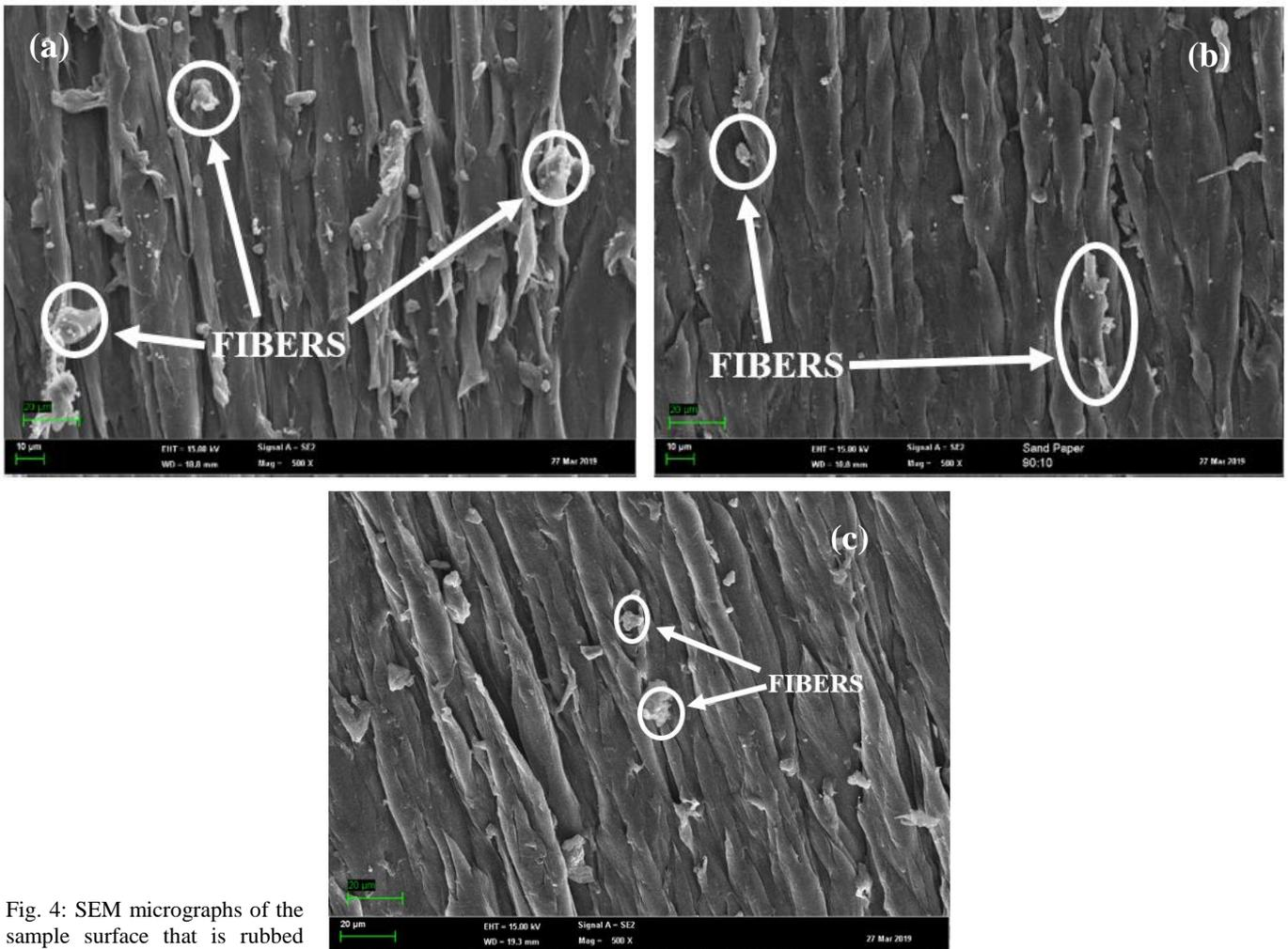
Fig. 4: SEM micrographs of the sample surface that is rubbed with sand paper (a)5wt% (b)10wt% and (c)15wt%
