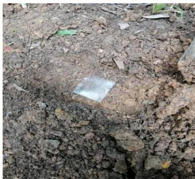
Fig. 13: Starch Bio-Based Plastic before Buried with 5cm Depth
