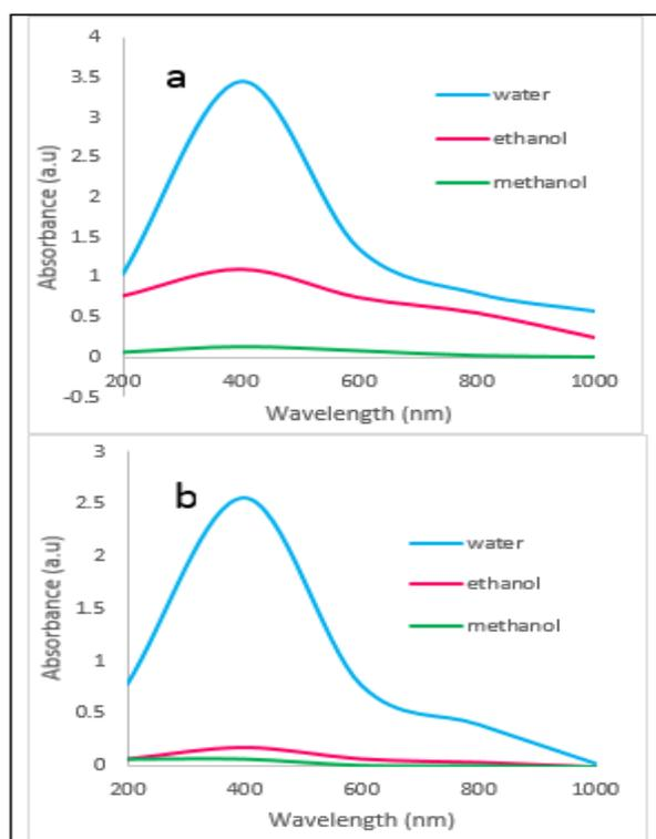
**Fig 5:** UV-vis absorption spectra of graphene oxide dispersed in different solvent (a) immediately after sonication and (b) left for one week (2 hour sonication time).
