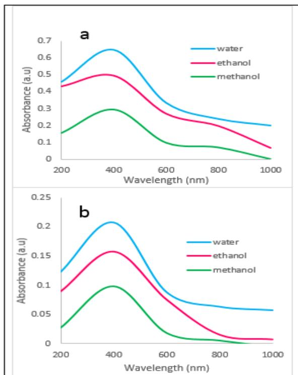
**Fig 4:** UV-vis absorption spectra of graphene oxide dispersed in different solvent (a) immediately after sonication and (b) left for one week (1 hour sonication time).
