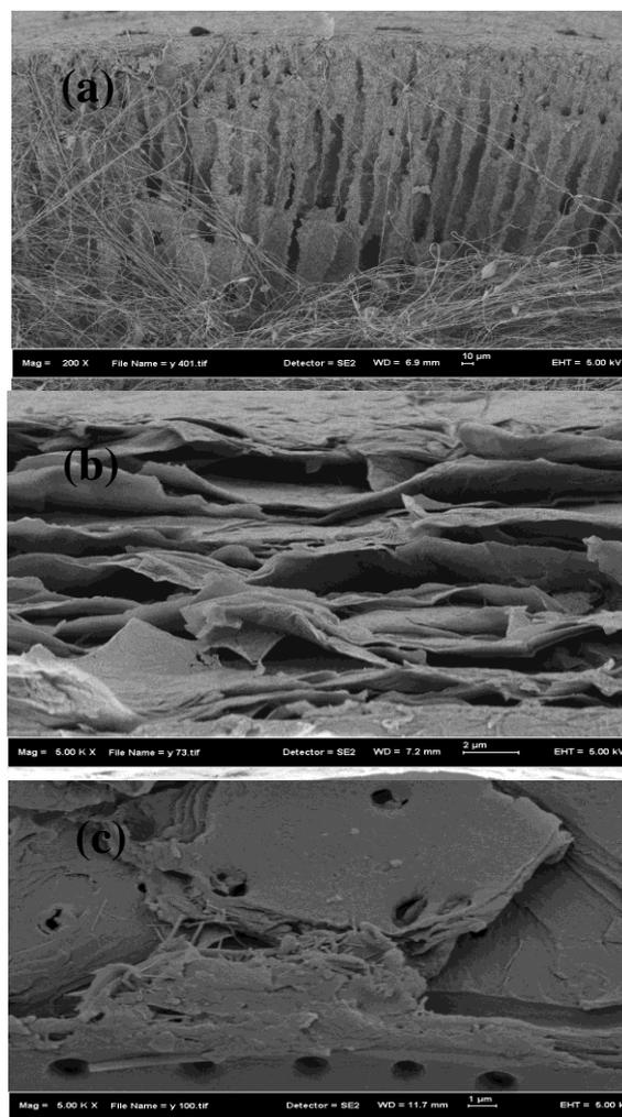
**Fig 1:** SEM image of graphene oxide (GO) at different size of microsphere range; (a) 10  $\mu\text{m}$  (b) 2  $\mu\text{m}$  and (c) 1  $\mu\text{m}$
