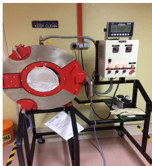
Figure 1 shows the Infrared Oven for VFIR drying
