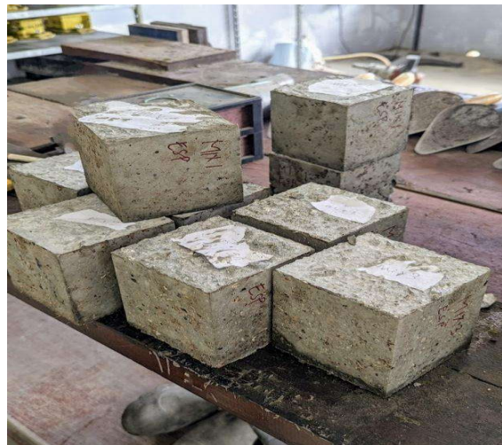
Figure.1 Precast Concrete Cube Sample with Eggshell Implementation
