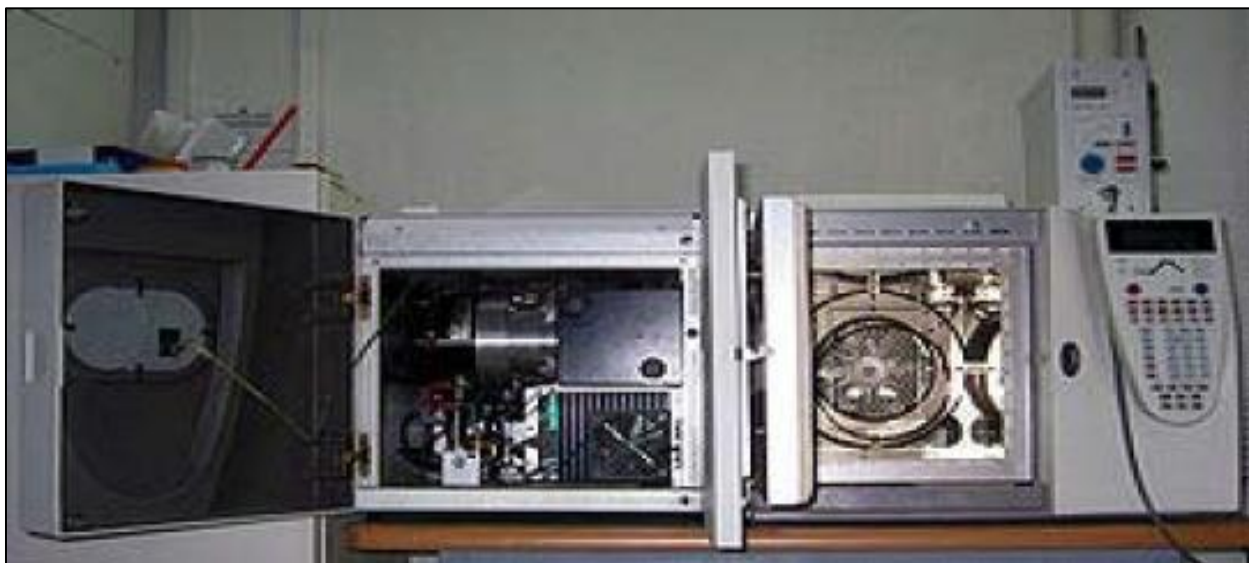
Figure 2.4: Insides of GC-MS looks like, with the gas chromatography column (Kataria Sahil et al. , 2011)
