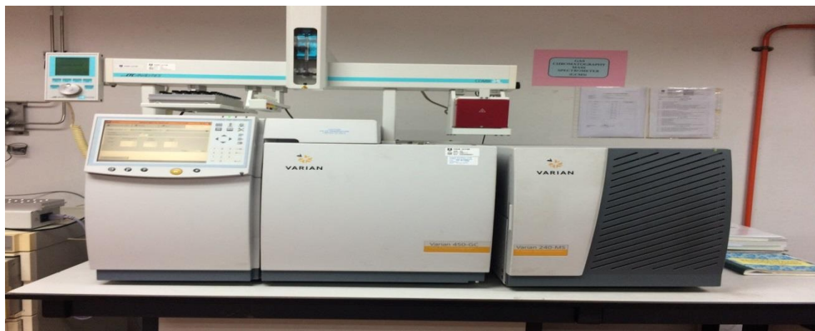
Figure 3.7: Gas Chromatographic-Mass Spectrometer (GC-MS) model Varian 240-MS completes with the 450-GC, with a Combi PAL autosampler from CTC Analytics
