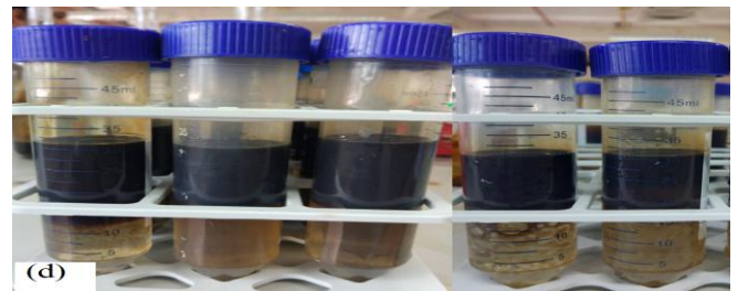
Fig.3: Demulsification bottle test (a) before separation, (b) 20:80 water cut emulsion, (c) 30:70 water cut emulsion, (d) 50:50 water cut emulsion after separation with addition of 40, 80, 120, 160, and 200 ppm graphene oxide from left tube to right tube.
