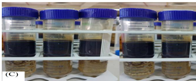
Fig.3: Demulsification bottle test (a) before separation, (b) 20:80 water cut emulsion, (c) 30:70 water cut emulsion, (d) 50:50 water cut emulsion after separation with addition of 40, 80, 120, 160, and 200 ppm graphene oxide from left tube to right tube.
