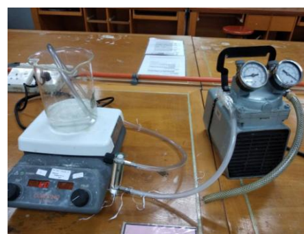
Figure 3 Induced air flotation (IAF) setup
