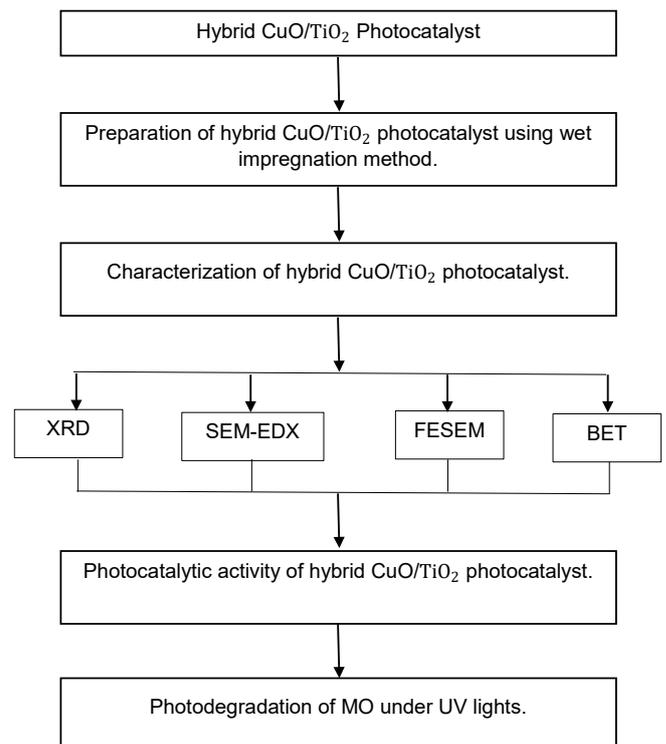
Fig. 3 : The overall process of the experiment.
