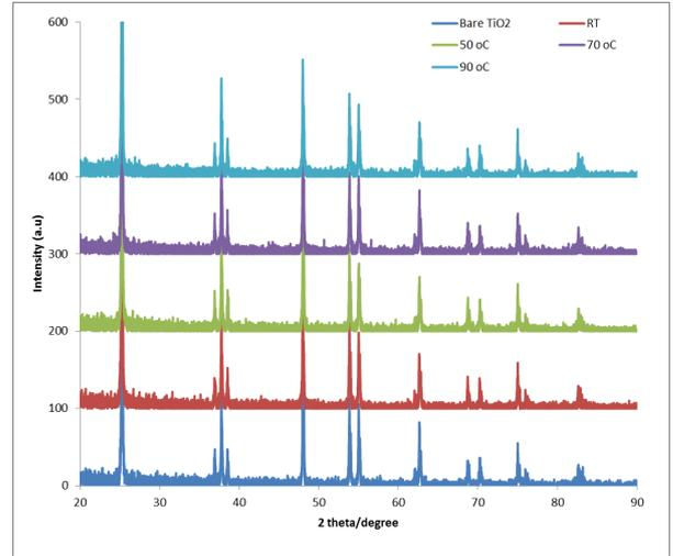
Fig. 4 : XRD pattern of the photocatalyst at different incubation temperature.
