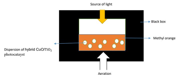
Fig. 2 : The experimental set-up of the photocatalytic activity.
