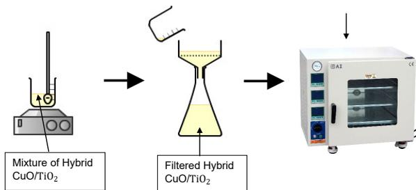
Fig. 1 : The experimental set-up of preparation process.
