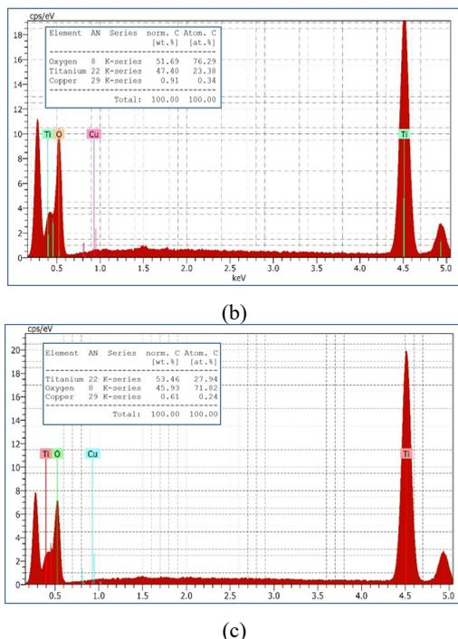
Fig.5 : The energy graph of (a) bare  $\text{TiO}_2$ , (b)  $\text{CuO}/\text{TiO}_2$  photocatalyst before degradation and (c)  $\text{CuO}/\text{TiO}_2$  photocatalyst after degradation.
