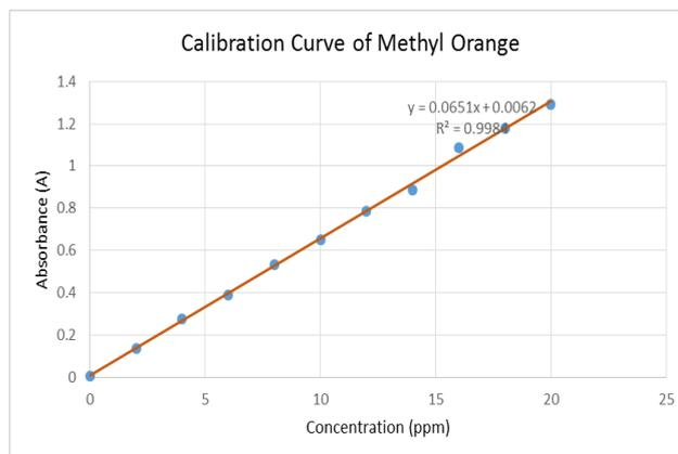
Fig. 12 : Calibration curve of Methyl Orange
