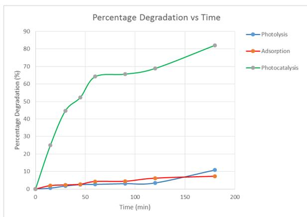
Fig. 11: Percentage degradation against the reaction time.
