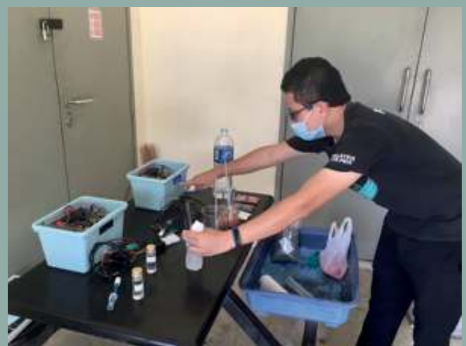
Figure 6.1 Soil NPK Sensor Calibration Process For AASAS
