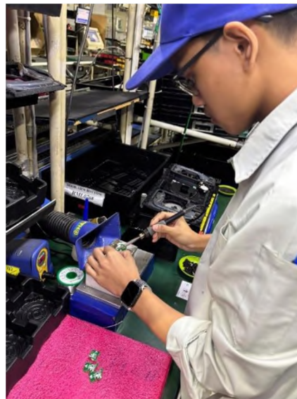
Figure 2.2 Soldering DC motor wire to PCB board
