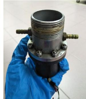
Fig. 6: Sonicator for sonication of POME
