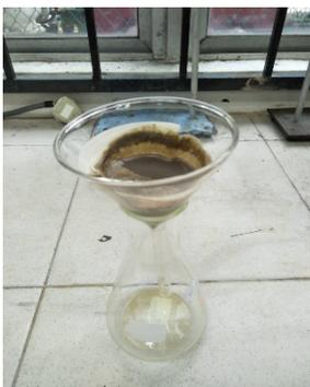
Fig. 4: Filter POME using filter paper.
