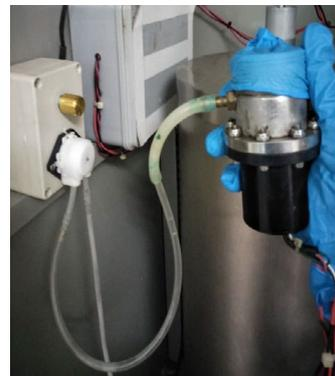
Fig. 7: Transfer of gas from sonicator into the gas bag by peristaltic pump
