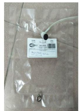
Fig. 8: Gas bag used to collect gas.
