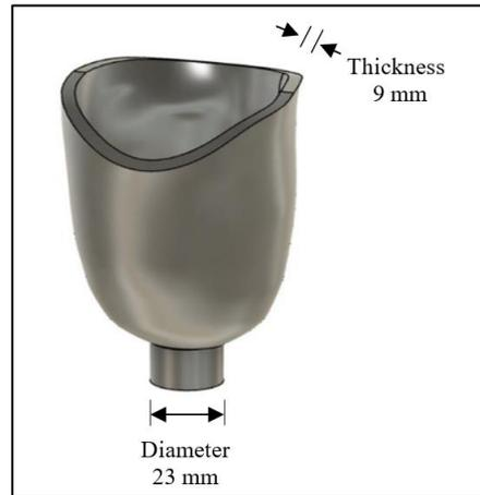
Fig. 4. Transtibial limb socket 3D model.
