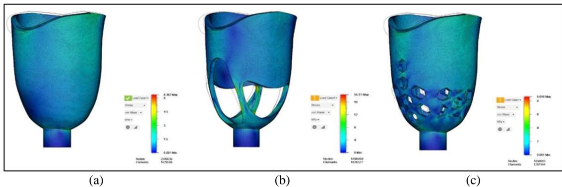
Fig. 8. Comparison of maximum stress distributions for three designs: (a) Design 1, (b) Design 2, and (c) Design 3.
