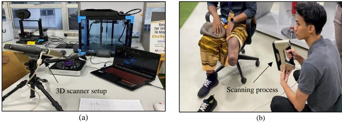
Fig. 2. Scanning session (a) 3D scanner setup and (b) scanning residual limb.
