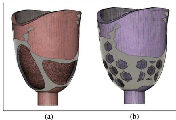
Fig. 6. Redesigning of transtibial limb socket using topology optimization (a) Design 2 and (b) Design 3.
