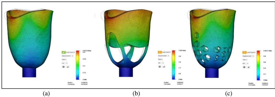
Fig. 9. Illustration of deformation results for (a) Design 1, (b) Design 2, and (c) Design 3, emphasizing differences in structural responses.
