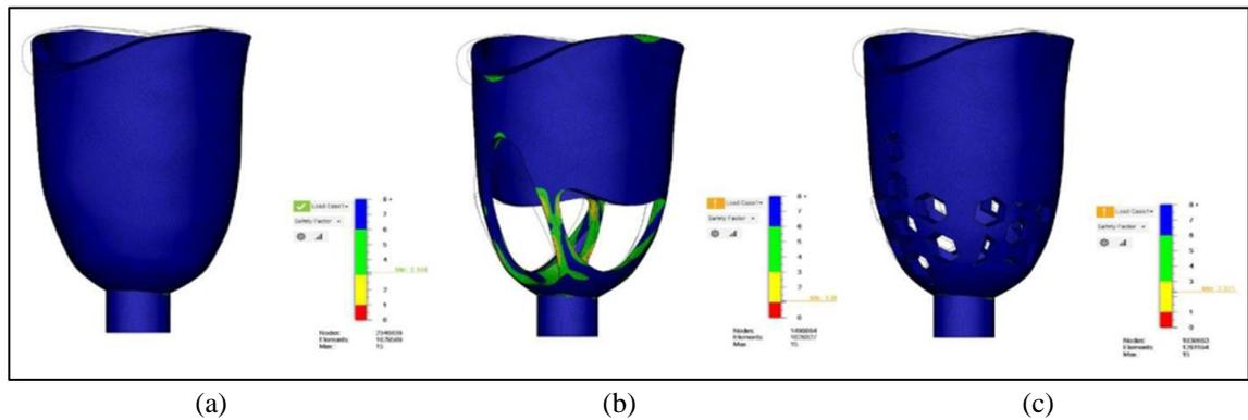
Fig. 10. Safety factor analysis results for the evaluated designs: (a) Design 1, (b) Design 2, and (c) Design 3.
