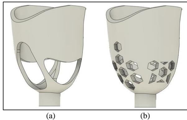
Fig.7. The revised model of transtibial limb sockets (a) Design 2 and (b) Design 3.
