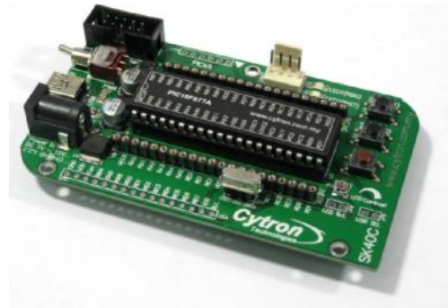
Figure 5 : A SK40C board with a PIC16F877A
