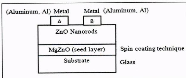
Figure 1. Illustration configuration layer of thin film
