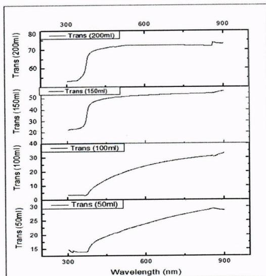
Figure 16. Optical transmittance of ZnO nanorods with different volumes of solutions
