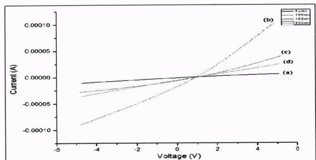
Figure 10. IV characteristics of ZnO nanorods for sample volumes at (a) 50ml; (b) 100ml; (c) 150ml; (d) 200ml
