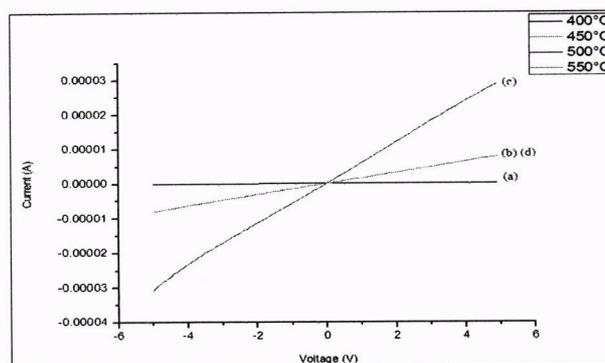
Figure 3. The IV characteristics of ZnO nanorods for sample annealed at (a) 400°C; (b) 450°C; (c) 500°C; (d) 550°C
