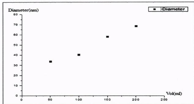
Figure 14. Diameter of the ZnO nanorods with different volumes of solutions
