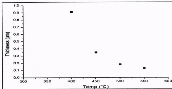
Figure 9. Thickness of the ZnO nanorods with different annealing temperature
