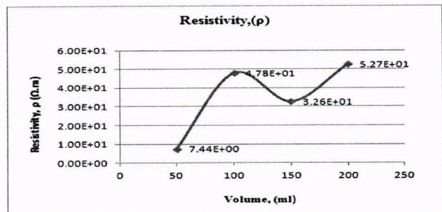
Figure 11. The measured value of resistivity of ZnO nanorods for all samples
