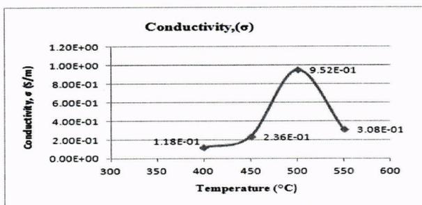
Figure 5. The measured value of conductivity of ZnO nanorods for all samples
