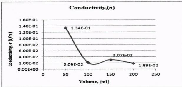
Figure 12. The measured value of conductivity of ZnO nanorods for all samples
