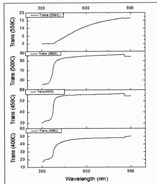
Figure 6. Optical transmittance of ZnO nanorods with different annealing temperature
