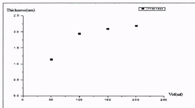
Figure 15. Thickness of the ZnO nanorods with different volumes of solution
