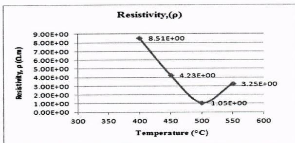
Figure 4. The measured value of resistivity of ZnO nanorods for all samples
