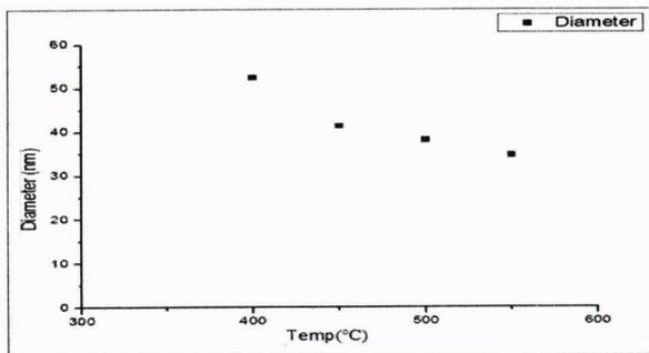
Figure 8. Diameter of the ZnO nanorods with different annealing temperature
