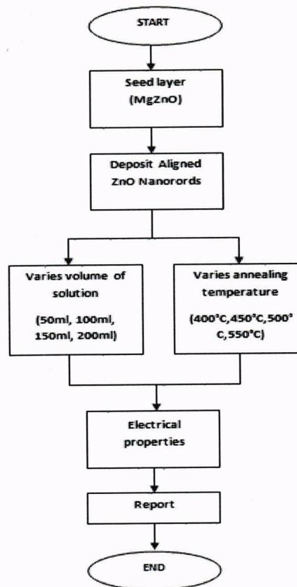
Figure2: Flow chart of the experimental procedure for the project
