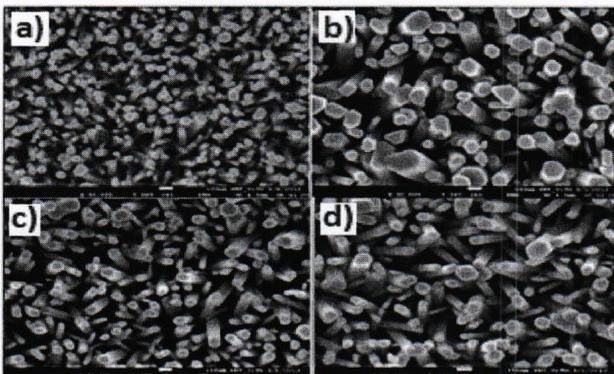
Figure 13. SEM images of ZnO nanorods of thin film: a) 50ml volume of solution; b) 100ml volume of solution; c) 150ml volume of solution; d) 200ml volume of solution
