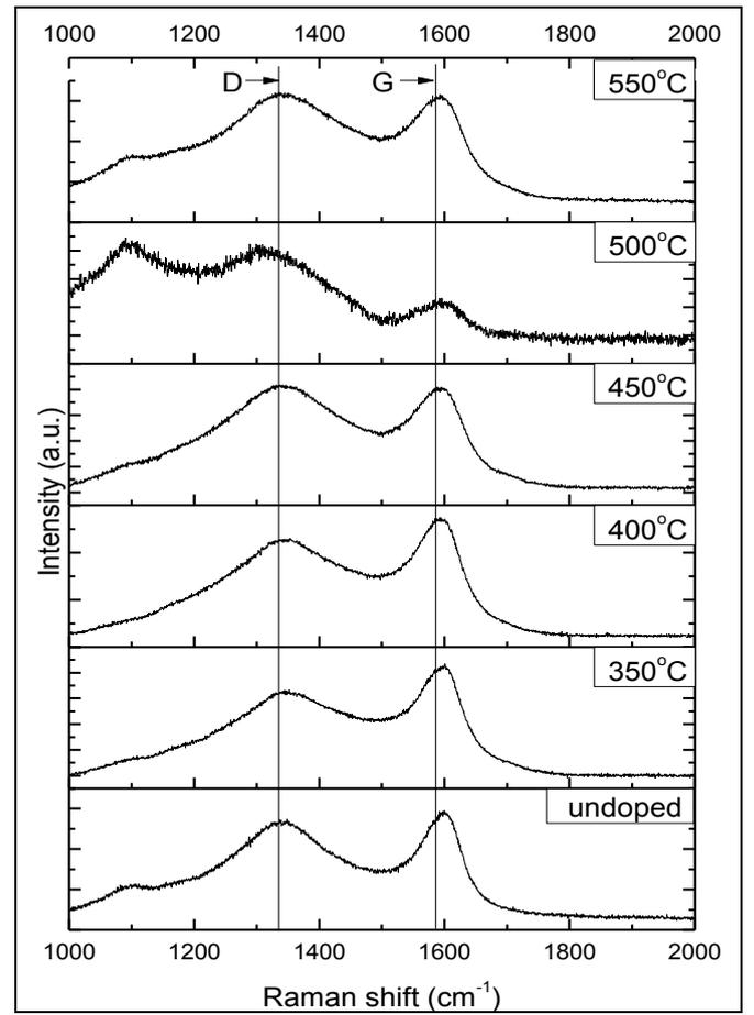
Figure 7: Raman spectra of a-C and a-C:I thin films doped at different doping temperature.
