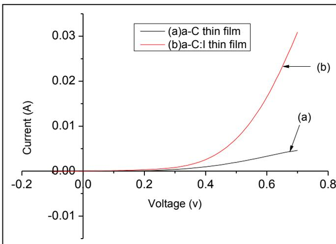
Figure 9: Solar cell graph of a-C and a-C:I doped at 450°C in dark
