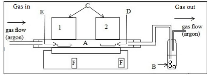
Figure 1: The schematic of CVD (A) Quartz tube (B) Water Bubbler system (C) Double furnace setup (D) Substrate (E) Combustion boat with camphor oil or iodine (F) Temperature controller
