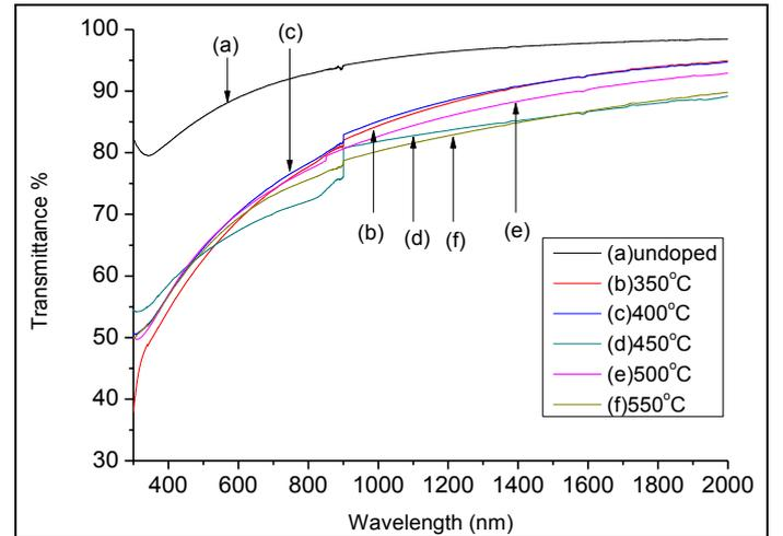
Figure 5: The optical transmittance versus wavelength of the a-C and a-C:I thin films doped at different doping temperature
