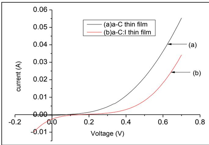
Figure 8: Solar cell graph of a-C and a-C:I doped at 450°C under illumination.
