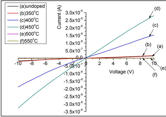
Figure 3: I-V curves of a-C:I thin films doped at different doping temperature under illumination condition.
