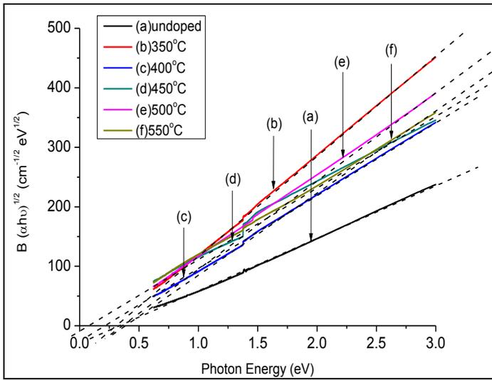
Figure 6: The Tauc plot as a function of photon energy ( $h\nu$ ) of the a-C and a-C:I thin films doped at different doping temperature.
