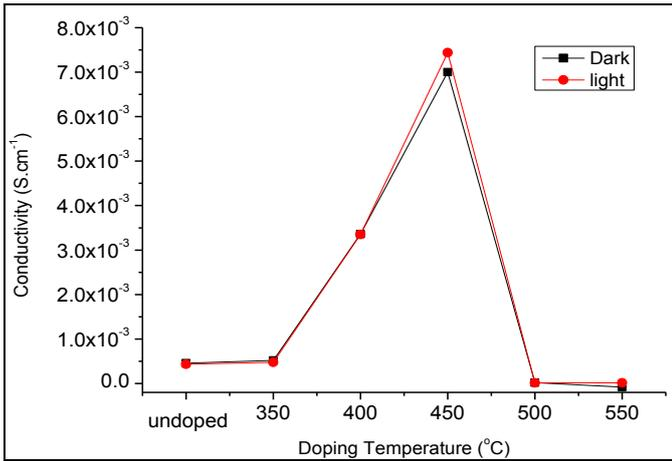
Figure 4: Conductivity of a-C:I thin films doped at different doping temperature
