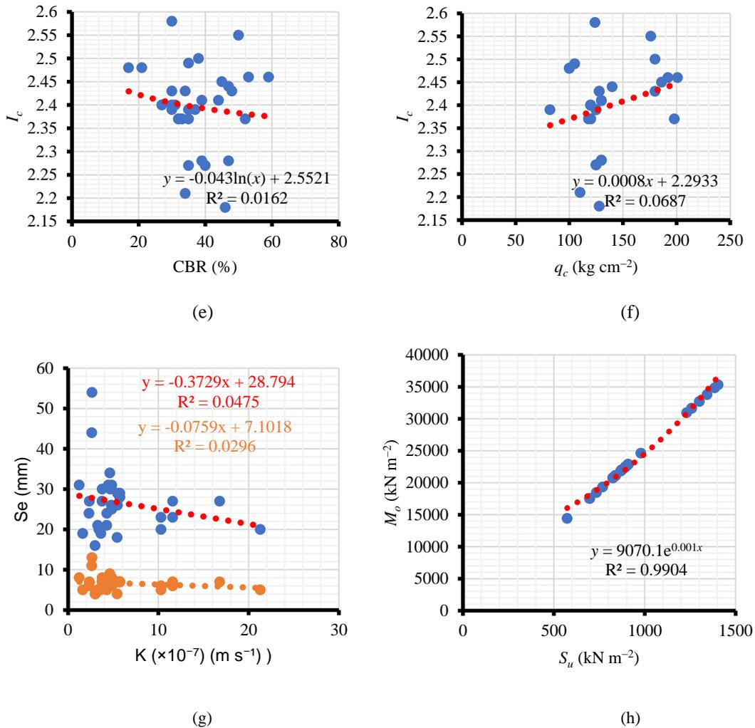
Fig. 4. Regression models for (a) CBR and  $M_o$  (b)  $R_D$  and CBR (c)  $S_u$  and  $q_c$  (d)  $\phi$  and  $q_c$  (e) CBR and  $I_c$  (f)  $q_c$  and  $I_c$  (g)  $K$  and  $S_e$  (h)  $S_u$  and  $M_o$ .
