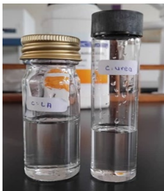
Figure 1: Eutectic mixture of ChCl: LA (left side) and ChCl: urea (right side).
