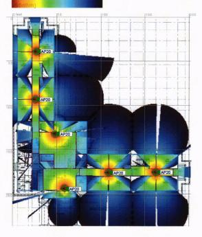
Fig.10- Estimation location for Access point with 5GHz band
