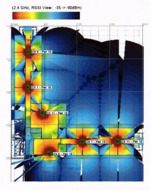
Fig.9- Estimation location for Access point with 2.4GHz band
