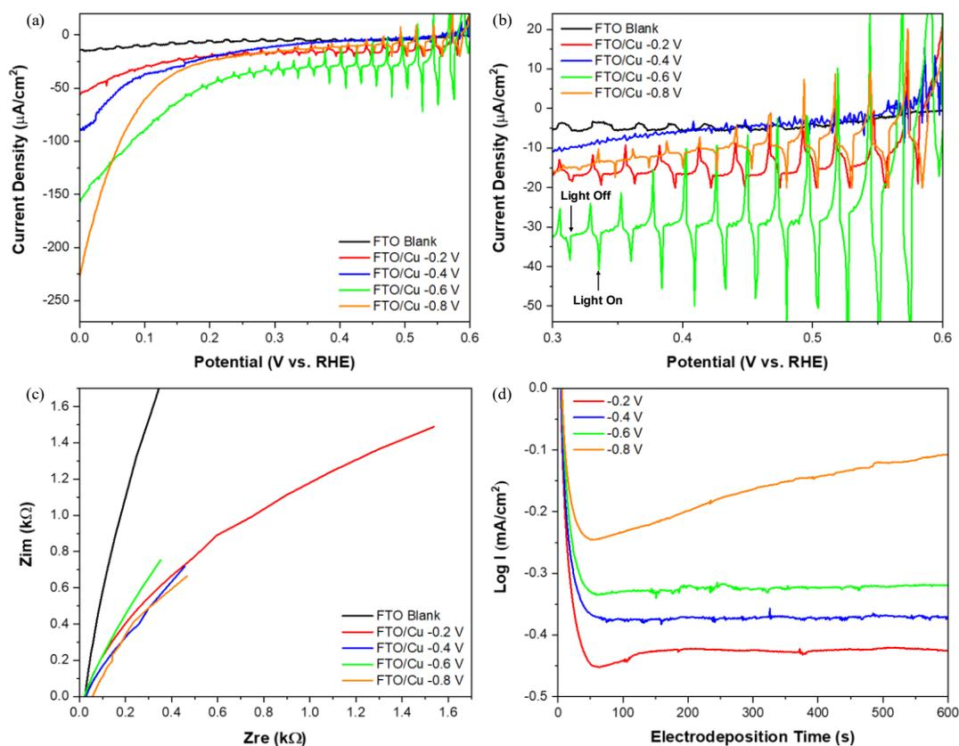
Fig. 3. (a-b) J-V curve of FTO/Cu with voltage range from  $-0.2 \text{ V}$  to  $-0.8 \text{ V}$  and its enlarged curve; (c) EIS plot, and (d) Log I vs. Cu ED time
