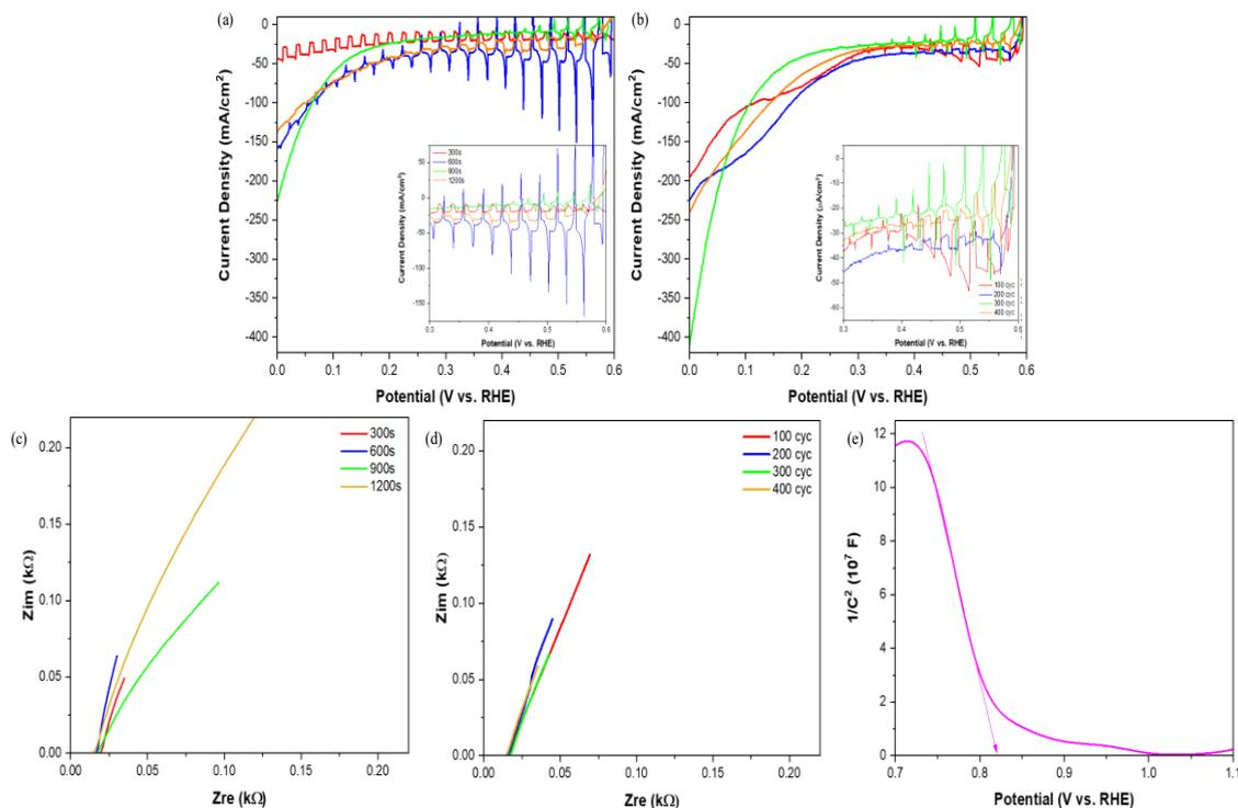
Fig. 4. J–V and EIS plot of FTO/Cu deposited via (a,c) DD, (b,d) PD, and (e) Mott-Schottky plot of the FTO/Cu
