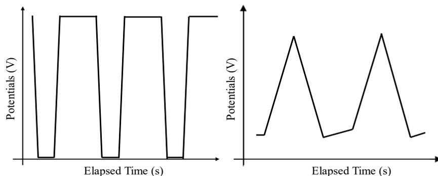
Fig. 2. Schematic representation of pulse electrodeposition (PD)
