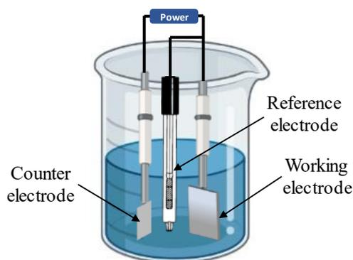
Fig. 1. Schematic diagram of ED method with three-electrode setup
