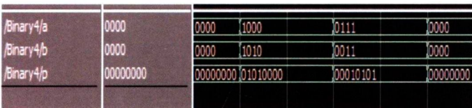
Fig 1.8 : Output waveform of 4-bit Array multiplier.
