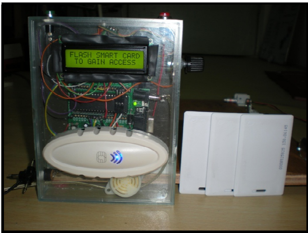
Figure 13: The completed housing of the security system
