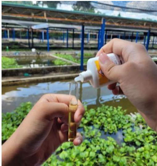
Fig. 5 On site ammonia measuring process using API ammonia test kit
