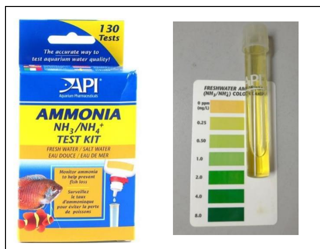
Fig. 1. API ammonia test kit with its colorimetric colour chart
