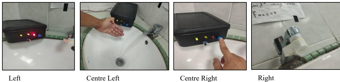
Fig. 2. Green, Yellow and Red Indicator Light with Red Switch On with mist spray installed (Left), Flow of water when IR Sensor Triggered without mist spray (Centre Left), Stop Push Button (Centre Right), Mist Spray Installed Zoom View (Right)
