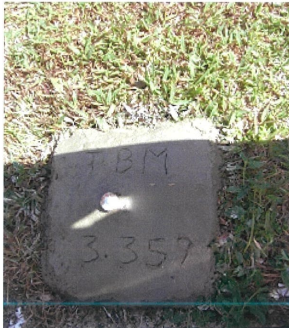
Figure 3.15: Temporary Benchmark (Source: Internet)
