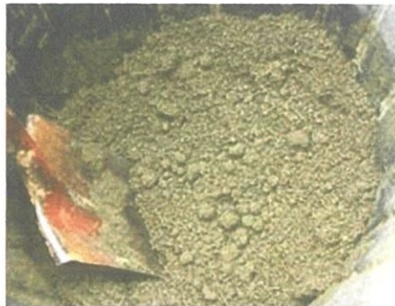
Photo 3.9 : Dry lean concrete
