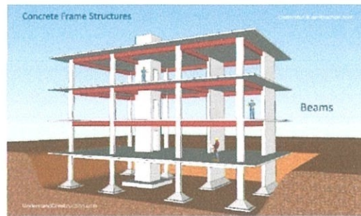
Figure 1.3 The beam structure in building (Source: UnderstandConstruction.com)
