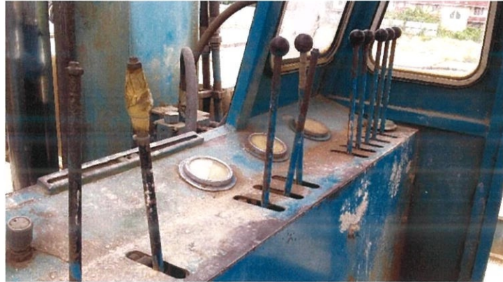
Figure 3.8 The control tools that use to stabilize the machine and jack in the pile.
