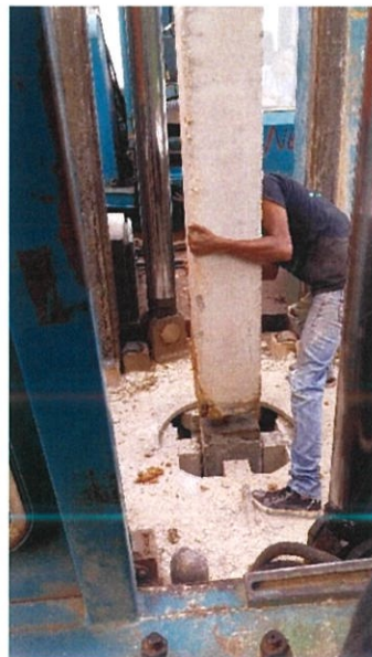
Figure 3.7 show the pile will put into the grip and the machine will grip the pile body.
