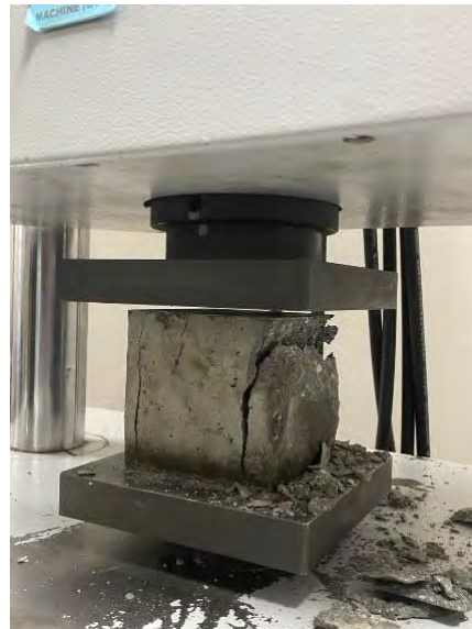
Figure 4: The concrete cube cracks after reaching its maximum load.
