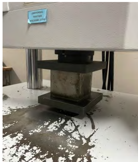
Figure 3: Place the concrete cube into a compressive test.
