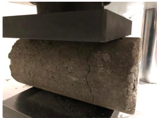
Figure 5: The concrete cylinder crack after reaching its maximum load.
