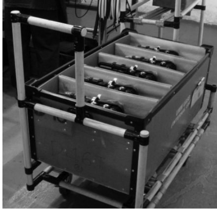
Figure 10: Finished Goods Trolley Used by Operator at Workstation 2
