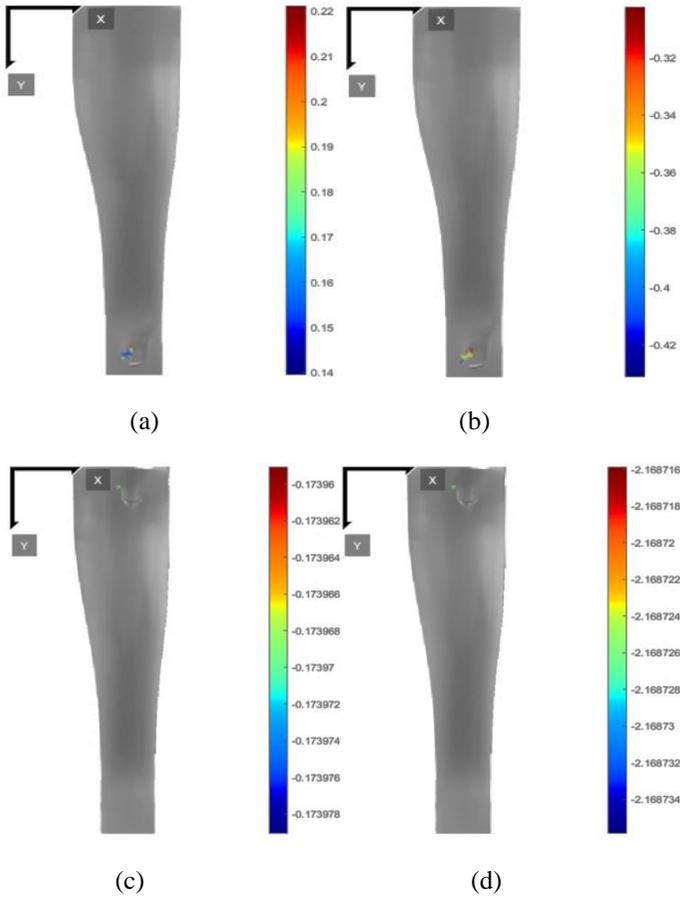
Figure 6: Lagrangian (a)  $\epsilon_{xx}$  strain (b)  $\epsilon_{yy}$  strain; Eulerian (c)  $\epsilon_{xx}$  strain (d)  $\epsilon_{yy}$  strain of blown film marked with spray paint
