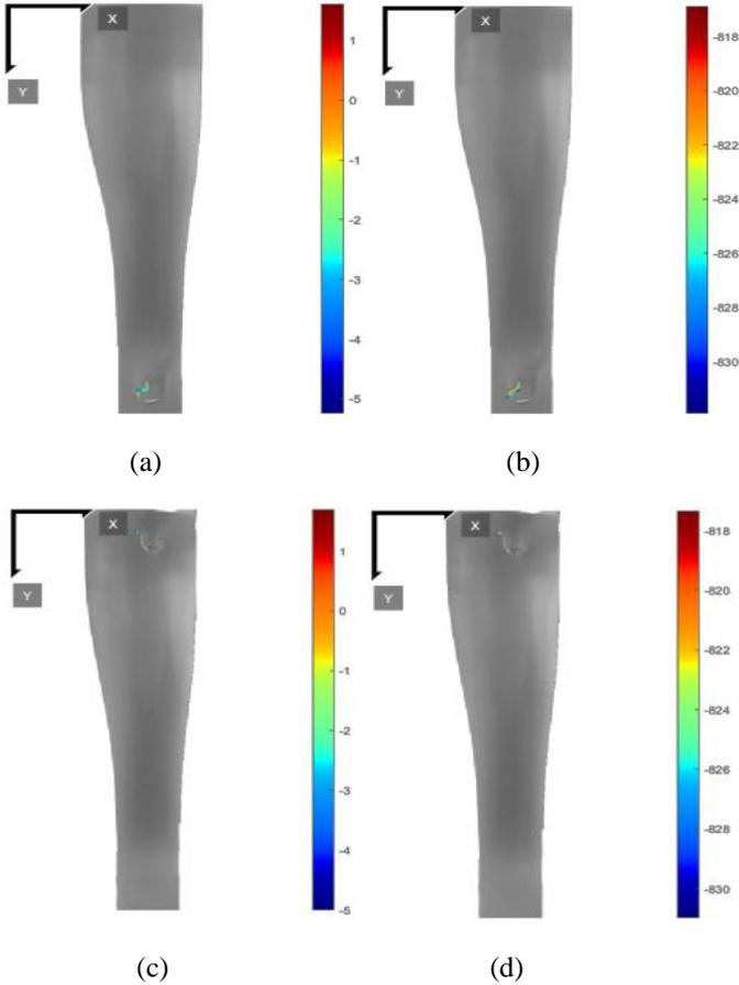
Figure 4: Lagrangian (a) u-displacement (b) v-displacement; Eulerian (c) u-displacement (d) v-displacement of blown film marked with spray paint
