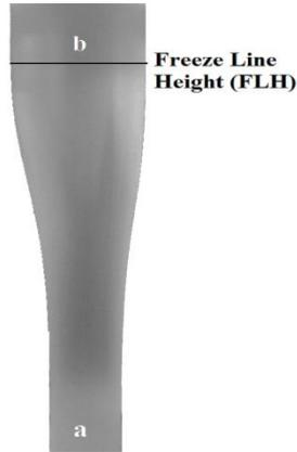
Figure 2: Position of blowing film (a) reference image (b) current image
