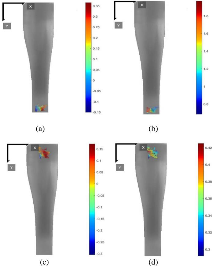
Figure 5: Lagrangian (a)  $\epsilon_{xx}$  strain (b)  $\epsilon_{yy}$  strain; Eulerian (c)  $\epsilon_{xx}$  strain (d)  $\epsilon_{yy}$  strain of blown film marked with marker pen
