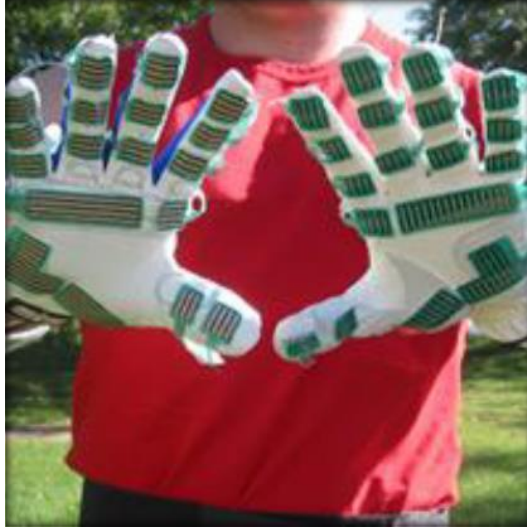
Figure 5: Eighteen sensors are attach to the glove
