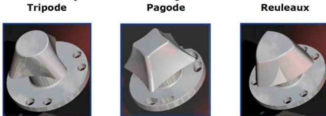
Figure 10: Mandrel shapes for non-circular spinning [4]
