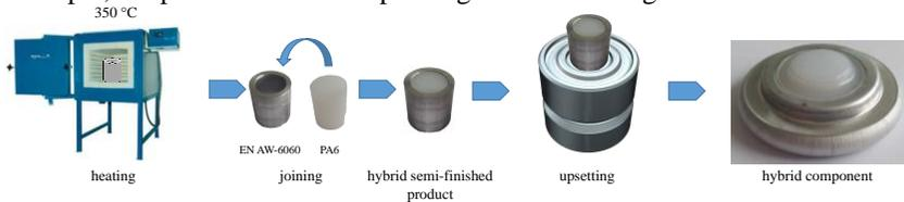
Figure 22: Process steps for the upsetting of hybrid aluminium-PA6 [16]
