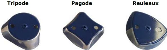
Figure 11: Components produced by non-circular spinning [4]
