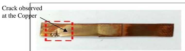
Figure 7. Crack at the Copper (Cu) substrate.
