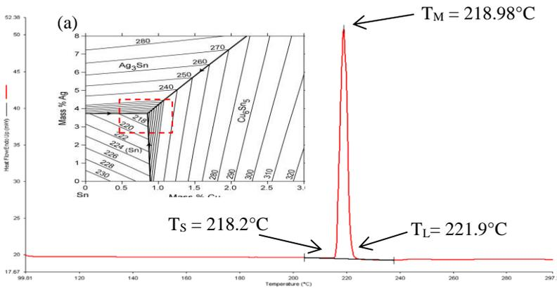
Figure 3. DSC result of SAC solder alloy, (a) Phase diagram of Sn-Ag-Cu.
