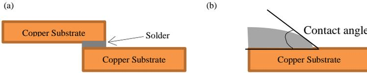
Figure 2. (a) Shear Test Specimen and Method and (b) Contact angle
