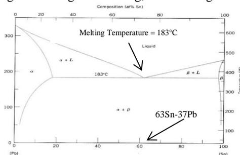
Figure 1: Phase Diagram of the Sn-Pb solder alloy.
