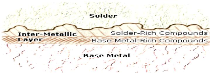
Figure 5. Solder/Substrate joint compounds representation.
