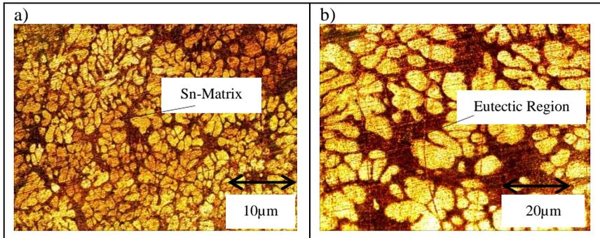
Figure 4: Microstructures of SAC solder alloy, (a) 10× and (b) 20×, magnification.
