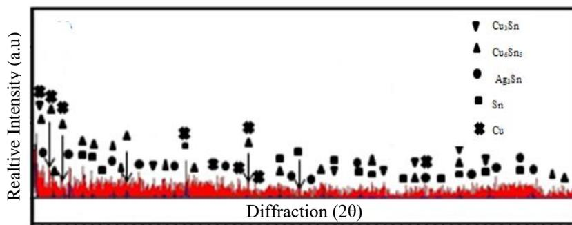
Figure 6. XRD of SAC solder alloy joint.
