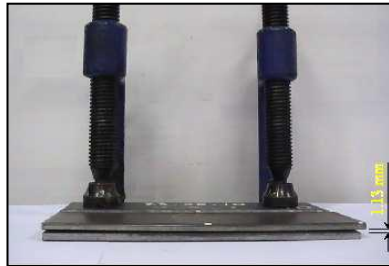
Figure 9: Angular distortion of specimen
