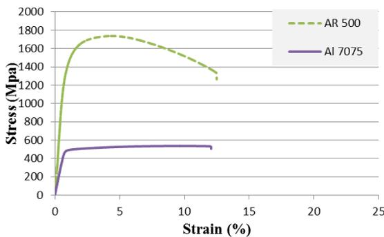
Figure 1: Stress strain curve for AR500 steel and Al7075
