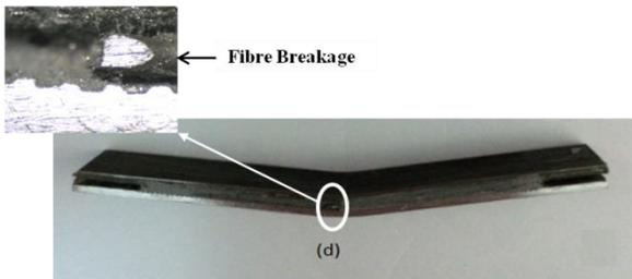
Figure 5: Fracture behaviour of metal composite laminate during bending test on (a) non-reinforced materials, (b) steel fibres, (c) wire mesh, and (d) fibre breakage
