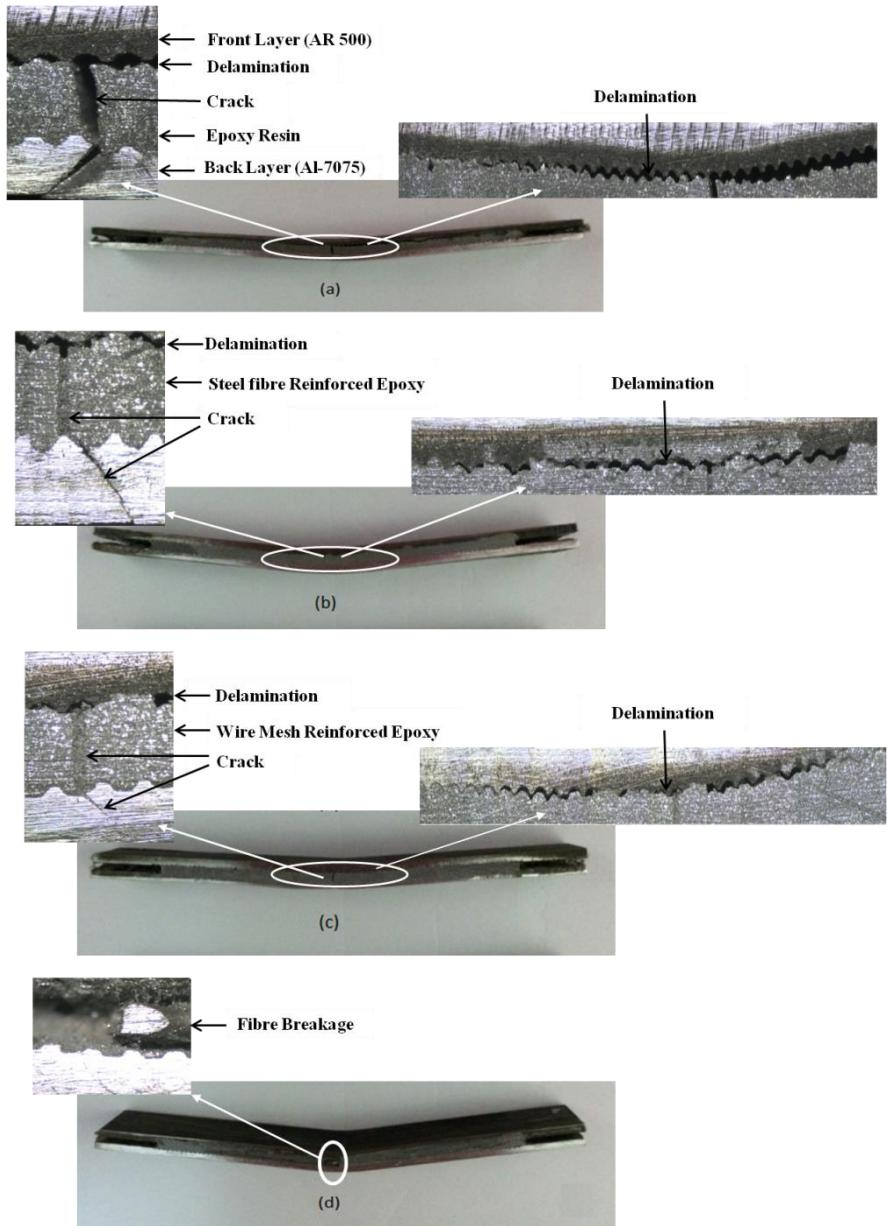
Figure 5: Fracture behaviour of metal composite laminate during bending test on (a) non-reinforced materials, (b) steel fibres, (c) wire mesh, and (d) fibre breakage
