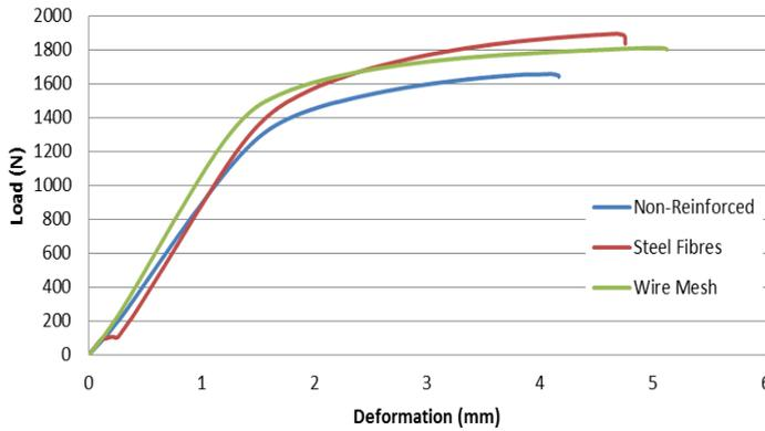
Figure 4: Load-deformation curves for non-reinforced, steel fibres reinforced and wire mesh reinforced composite laminate materials
