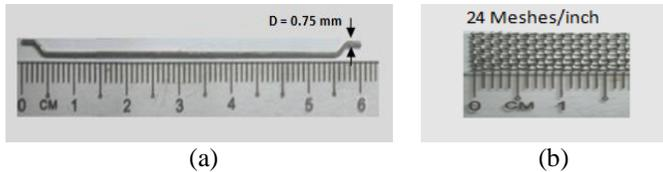
Figure 2: Geometry (a) Steel fibre and (b) stainless steel wire mesh used for reinforcement materials
