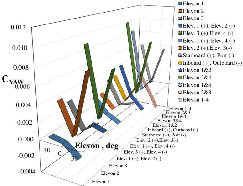
Fig. 9: Yaw coefficient versus deflection angle
