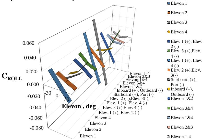
Fig. 7: Roll moment coefficient versus deflection angle
