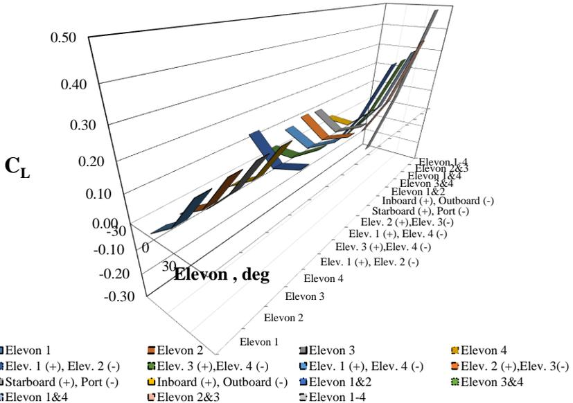
Fig. 6: Lift coefficient versus deflection angle
