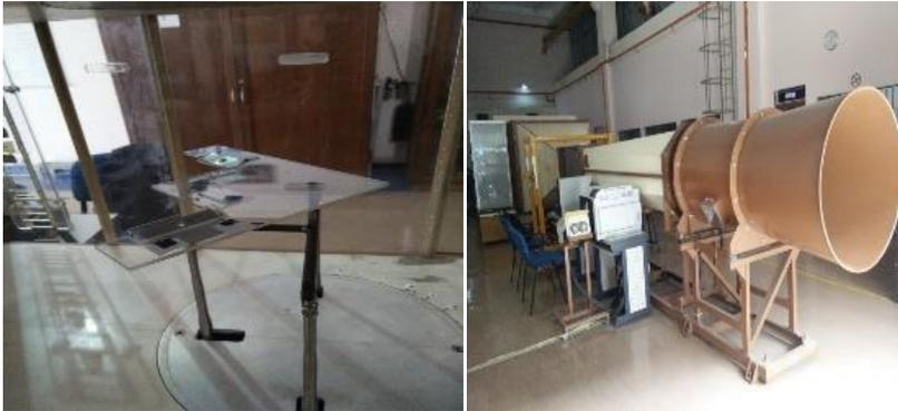
Fig 3: BWB model mounted inside the wind tunnel chamber (left) and Low Speed Wind Tunnel (LST-1) at FTTC, UiTM (right)
