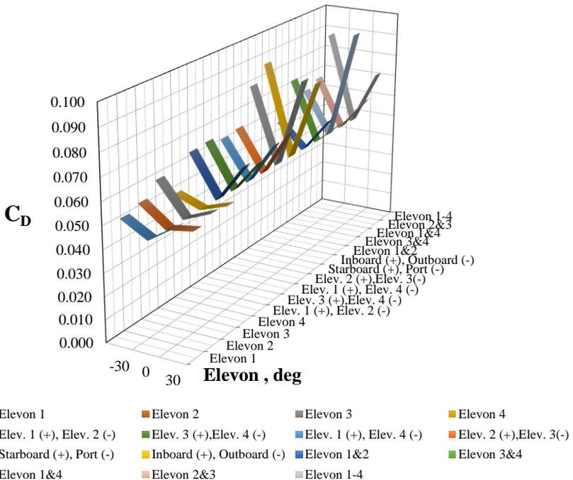
Fig. 4: Drag coefficient versus deflection angle
