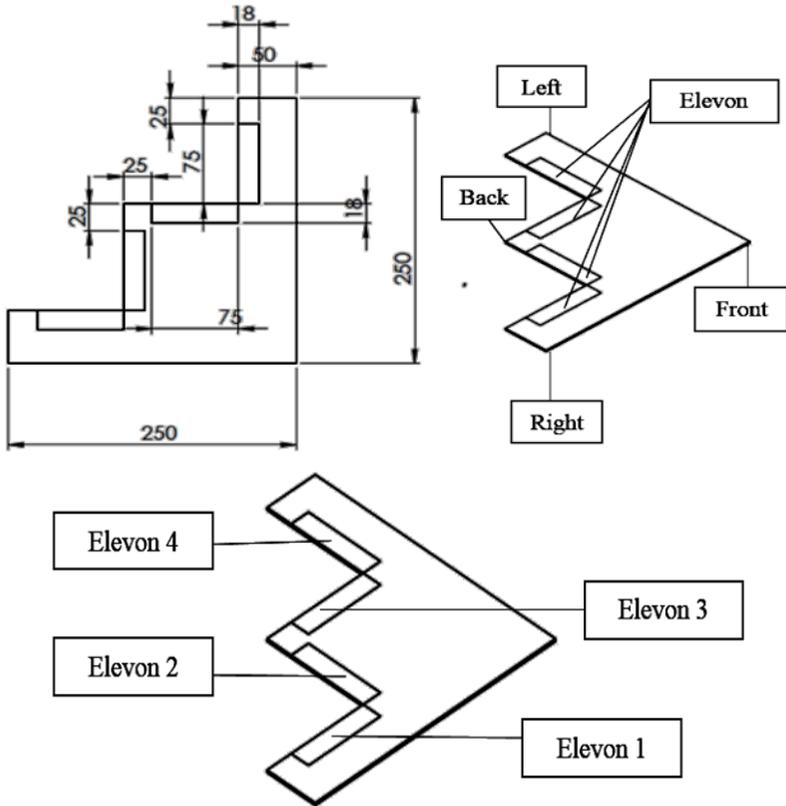
Fig. 2: Dimension of BWB flat model in mm unit and numbering of elevons
