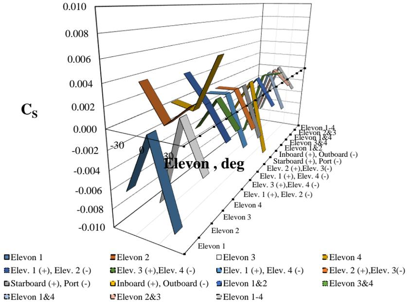
Fig. 5: Side force coefficient versus deflection angle
