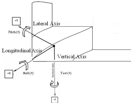
Fig.1 The body axes of the aircraft.
