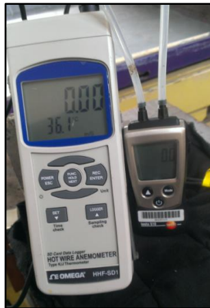
Figure 4: Hot wire anemometer and Testo 510 for the pitot-tube
