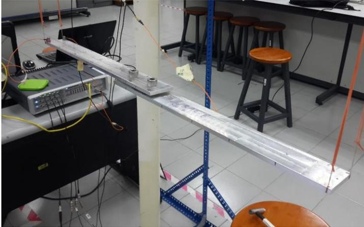
Figure 5: Experimental modal analysis setup
