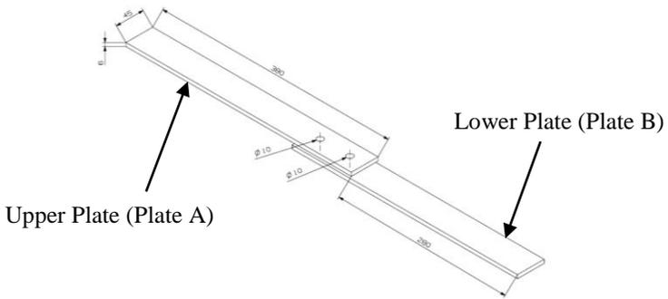
Figure 1: Geometry of the bolted lap joints
