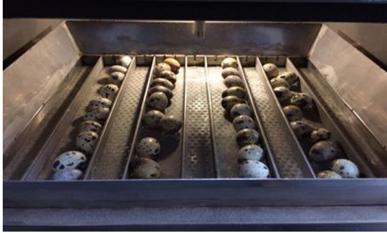
Figure 4: Eggs placement using 360° rolling mechanism
