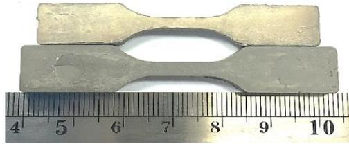
Figure 4: Compact dimensional difference between the green compact (below) and the sintered compact (upper)
