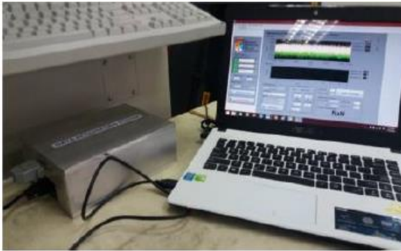
Figure 2: Neo MoMac cutting force measuring system
