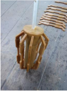
Figure 3: Wax pattern tree
