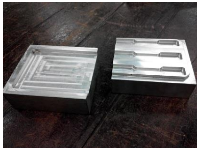
Figure 1: Tensile test specimen mold
