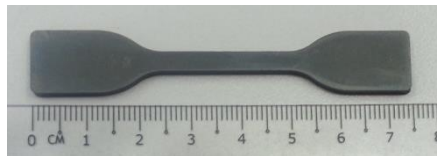
Figure 5: Injected feedstock with tensile shape design (green part) without physical defects
