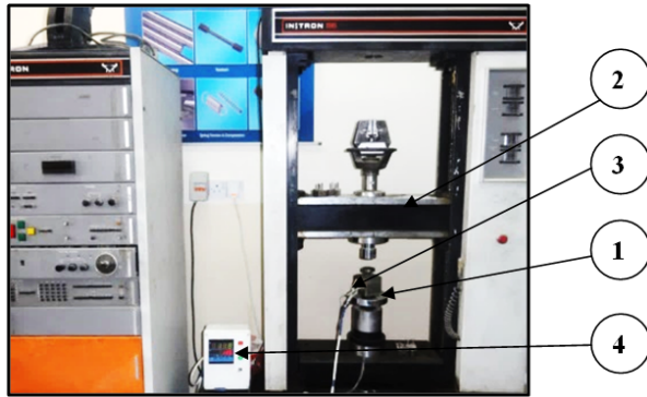
Figure 1: The fabricated hot pressed systems (1), installed on the Instron testing machine (2); thermostats (3) connected to the digital temperature control system (4)
